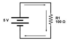
Here, we have one 5-volt voltage source in series with one resistor R1 with a resistance of 100  $\Omega$ . Because we have only one resistor, the total voltage across it will be equal to the voltage of the source, 5 V. We can now apply Ohm's law to find the current in the circuit:
