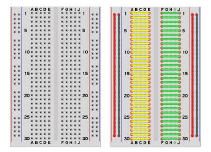
On the left we have a simple breadboard; on the right, we have the same breadboard with the internal connections shown. At the bottom and the top of the board we can see letters. If we follow, we can see that, on each row, the letters **A**, **B**, **C**, **D**, and **E** are interconnected, as shown by the yellow wire.
