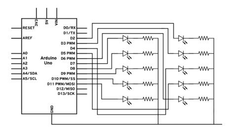
Here is one possible way of wiring it on a breadboard:
