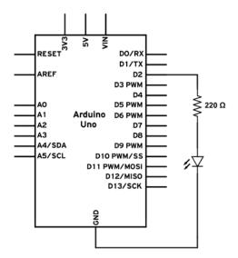
Here is a simple way of wiring the LED:
