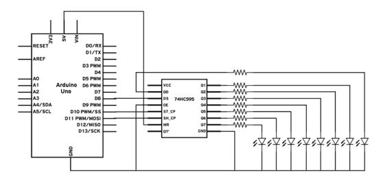
Here is an example of how to wire it on a breadboard:
